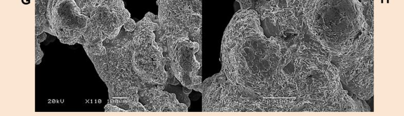
supplied by the manufacturer G and H) SEM images of the porous TiAl6V4 material revealing a rough surface.
