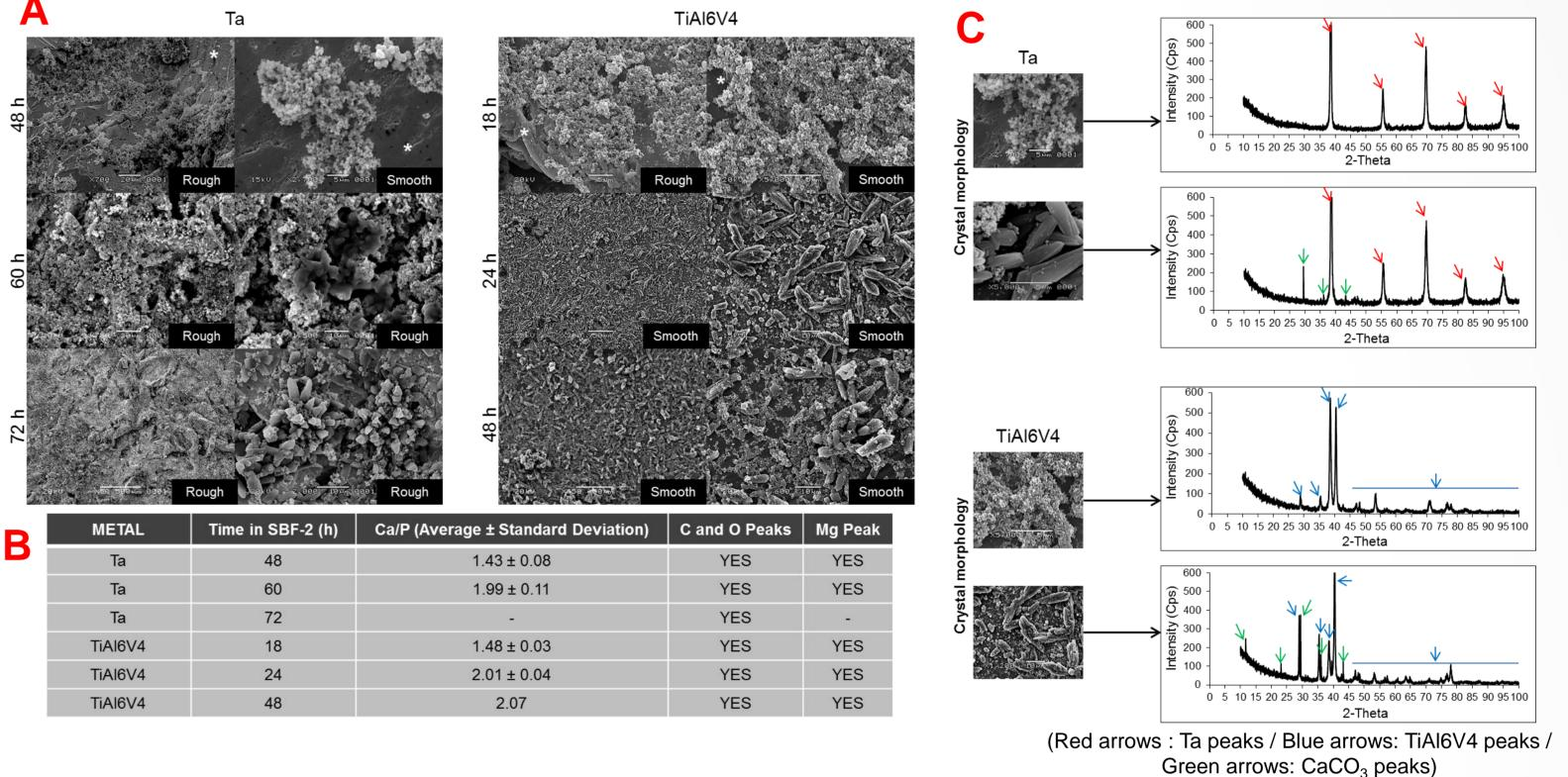
Prediction of *in vivo* behaviour (immersion in SBF) showed that the CaP deposits would act as a catalyst to rapidly form a Ca deficient CaP layer that also incorporates Mg demonstrating their bioactivity (D).
